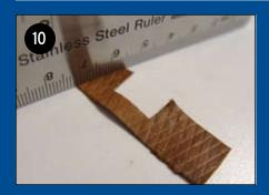
Left: Place the metal ruler edge-down on the leather. Tap it with the hammer two or three times; don't hit too hard or you can cut the hide. Make sure the lines are evenly spaced.
