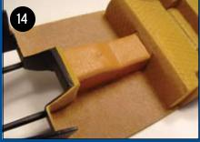
Working from the bottom up helps conceal gaps. I covered the driveshaft tunnel first, then applied flocking, which covers the seams between the leather and the floor. The leather that will go on the rear seat will hide the tunnel's rear seam.
