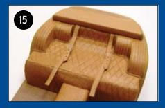
Left: After the panels are installed, burnish the seams with a fine burnishing tool or a smooth, round toothpick. If needed, make piping from thin wire and run it over the seams. The more leather detail you add, the better your model's interior will look.
